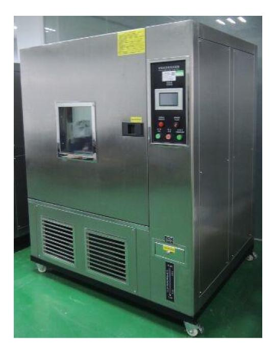
800 L Programmable Temperature & Humidity Chamber is designed for testing the capability of heat-endurance, cold-endurance, dryness-endurance, and humidity-endurance,
